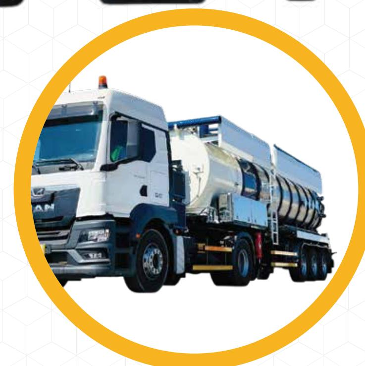
The IVT POWERVAC LTS is specifically designed for suction, transporting, and unloading of liquid and hazardous substances such as liquids, sludge, fats, oils, fuels, and chemicals in the (heavy) industry. This robust machine operates gently with a 2500m<sup>3</sup>/h liquid ring vacuum pump. Specially developed for working with hazardous and contaminated substances, the truck is available in ADR/API 2219 versions and built-in accordance with all applicable safety standards.
