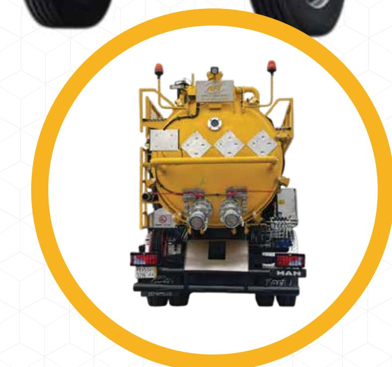
The IVT BLOWVAC is specifically designed for suction, transporting, and unloading of liquid and hazardous substances in the (heavy) industry. This robust machine operates gently with a 3600m<sup>3</sup>/h air injection vacuum blower. The mechanical level indicator with a float ball warns timely which makes it possible to empty the hoses without spilling any fluids. The cyclone filter clears the airflow from any carried along residue which keeps the filtration system clean.
