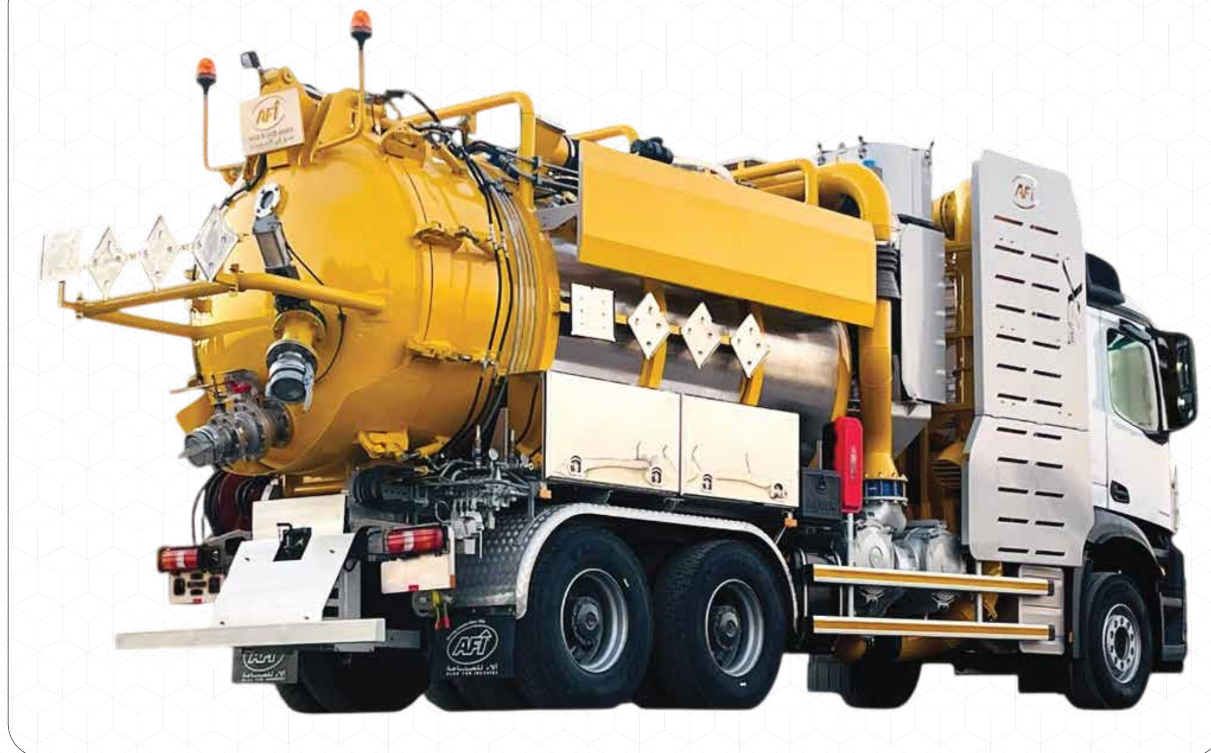
The IVT X-VAC Industrial Vacuum Loader with cyclone separation technology is engineered for demanding industrial applications. It is designed to suction, displace (optional), transport, and discharge a wide range of dry, wet, and hazardous materials, including catalysts, gravel, powders, cement, phosphate, fly ash, and sludge.
